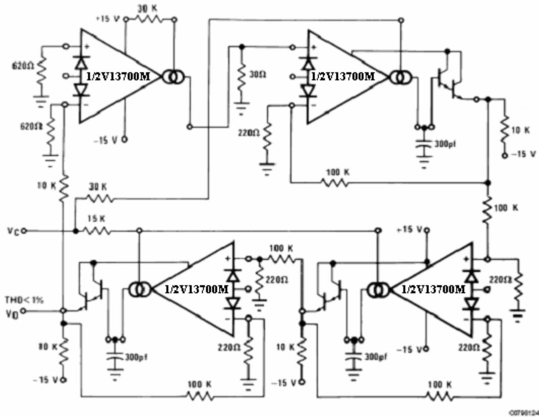
FIGURE 17. Sinusoidal VCO
